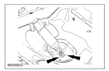
3. **NOTE:** Before installation, make sure the safety belt webbing is not twisted and the safety belts and buckles are accessible to the occupants.
